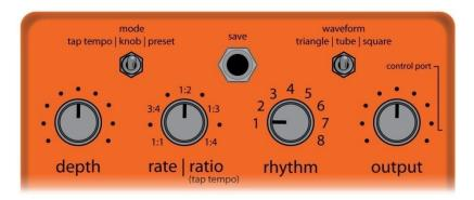
Plug your guitar into the lower jack on the right side. Plug your amplifier into the jack on the left side. Plug a  $9-12V_{DC}$  power supply into the power jack on the left side (2.1mm barrel connector, negative tip). Set the mode switch to "knob," the waveform switch to "tube," the depth to half, rate to half, rhythm to 1, and output to half.
