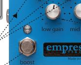
**Boost Stompswitch:** Toggles on/off the boost section of the unit. When the LED is shining, the boost is applied to the signal.
