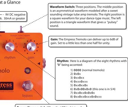
**Bypass Stompswitch:** When the LED is shining, the tremolo effect is applied to the signal. When off, the tremolo is being bypassed (true bypass).
