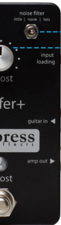
**noise filter:** Select the amount of filtering applied to pedals in the loop.
