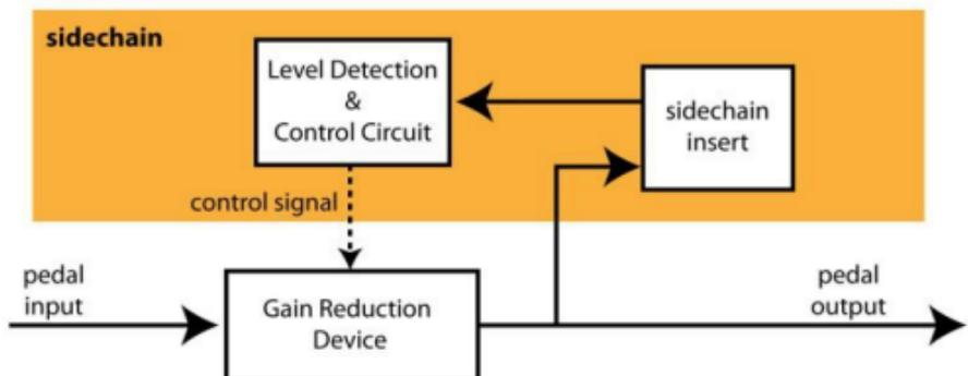
**input:** sets the level entering the compressor circuit. Higher levels result in more compression.
