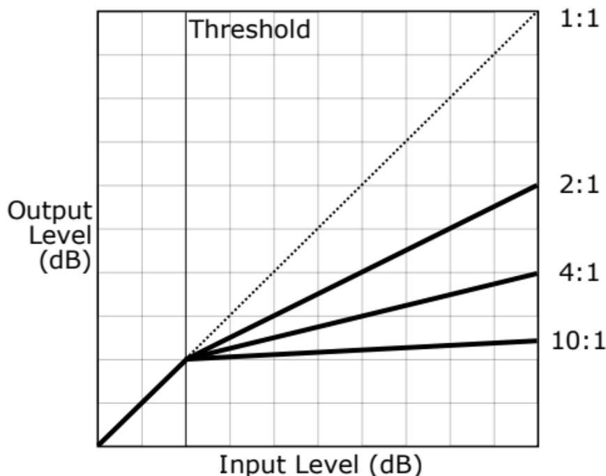
The **ratio** determines how much gain reduction will be applied to the signal once it crosses over the threshold. At a 4:1 ratio, for every 4dB of input signal above the threshold, there will be 1dB of output signal. A 10:1 ratio would output 1dB for every 10dB of input signal, etc.
